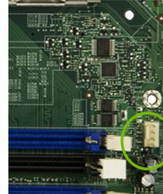
Note that the CPU fan cable can be either a 3-pin or a 4-pin connector. Connect a 3-pin connector to pins 1, 2, and 3 on the motherboard connector.
