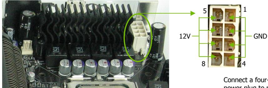
Connect a four-pin power plug to pins 1, 2, 5, and 6.
