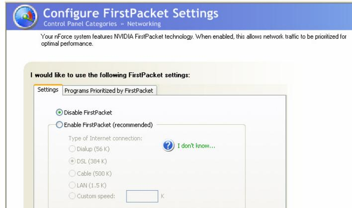
3. Click **Enable FirstPacket (recommended)** to enable the options that define the speed of the broadband connection. This information is needed by the FirstPacket software to appropriately prioritize network traffic.
