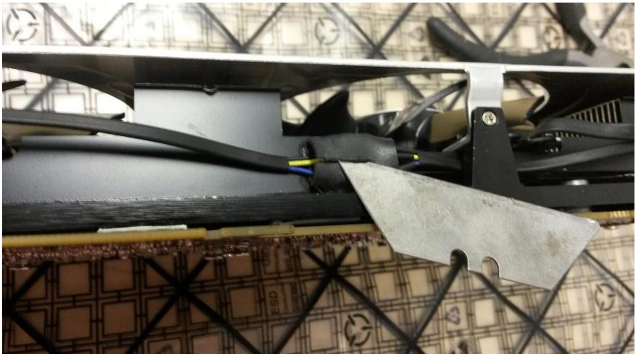
Then delicately separate the clips. Be careful not to pull the wires on this step, this particular plastic union is less durable than the clip in the PCB of the video card and can be damaged easily. It's okay to slowly jostle them free, however, some clips are very tight and require tools (like a razor blade or needle nose pliers).
