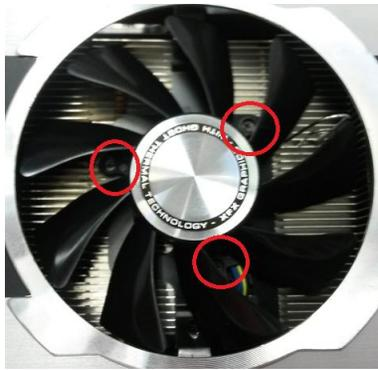
Then, take a sharp razor blade, and gently cut a slice through the protective sleeve on the fan connectors.
