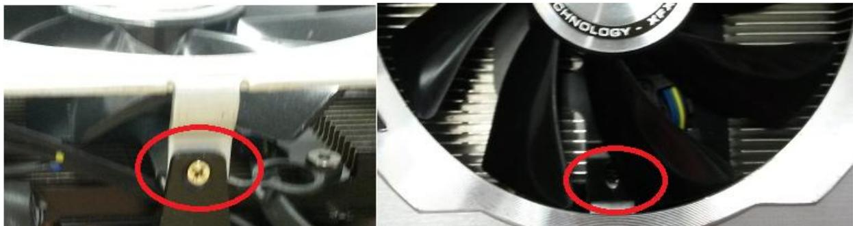
In order to remove the cables from the card, you have to remove two screws on the rear fan. The side screw (pictures above left) and the mount screw (above right) which are nearly an inch apart. Removal of these screws is needed to bend the metal inwards (toward the fan, so you can slide the cable out).
